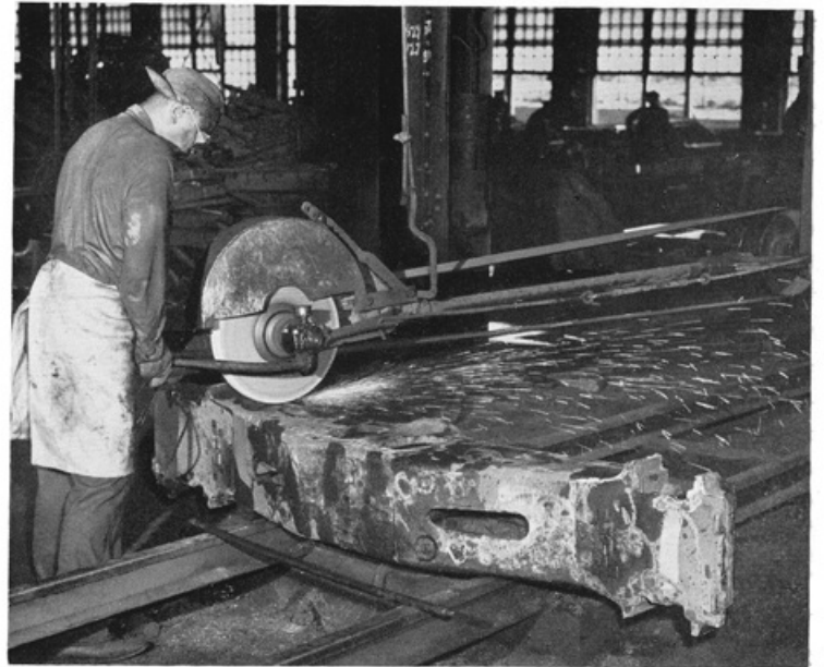
Grinding Bolster. Various types of grinders are used to smooth objectionable rough spots.
