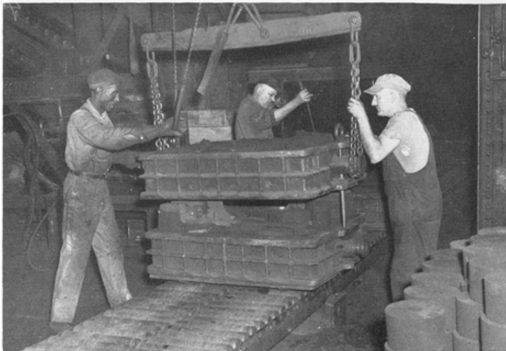
At this station the cope joins the drag to complete the mold. Clamps are applied to secure the cope to the drag and the mold is ready for transfer to the pouring floor.
