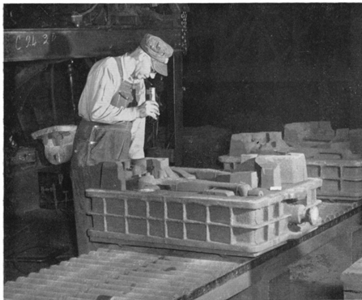
Cores have now been set in the drag, and careful inspection follows.
