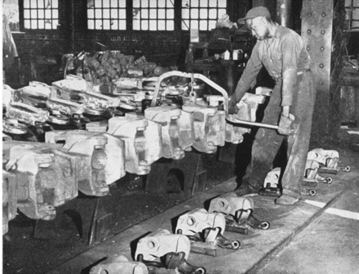
Fitting Coupler. — In this operation the knuckle, lock, thrower, pin, and operating linkage are assembled into the coupler body, and tested for proper operation.
