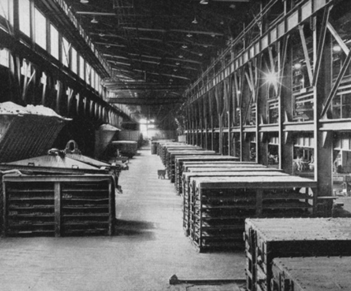
Looking west in the Transportation Bay. This extends the full length of the molding section of the Foundry. A number of loaded core racks may be seen, located adjacent to the molding stations.
