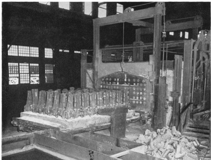
Here we see an annealer load of coupler bodies which have just been taken out of the furnace in the immediate background.
