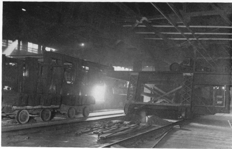
Charging scrap into one of the melting furnaces. Six hours are normally required to charge, melt, refine, and tap a heat of steel.
