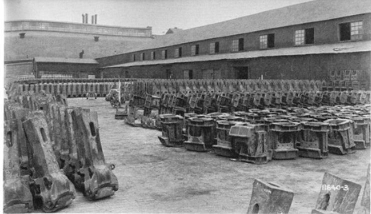
A section of the Shipping Platform showing couplers and various draft castings awaiting shipment.
