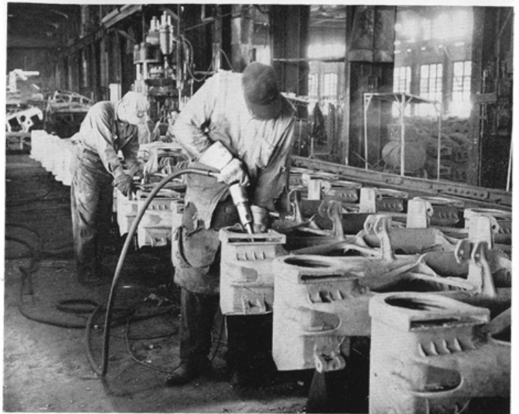
Chipping Truck Side Frames. Air-hammers using hardened steel chisels are used in this important finishing operation.
