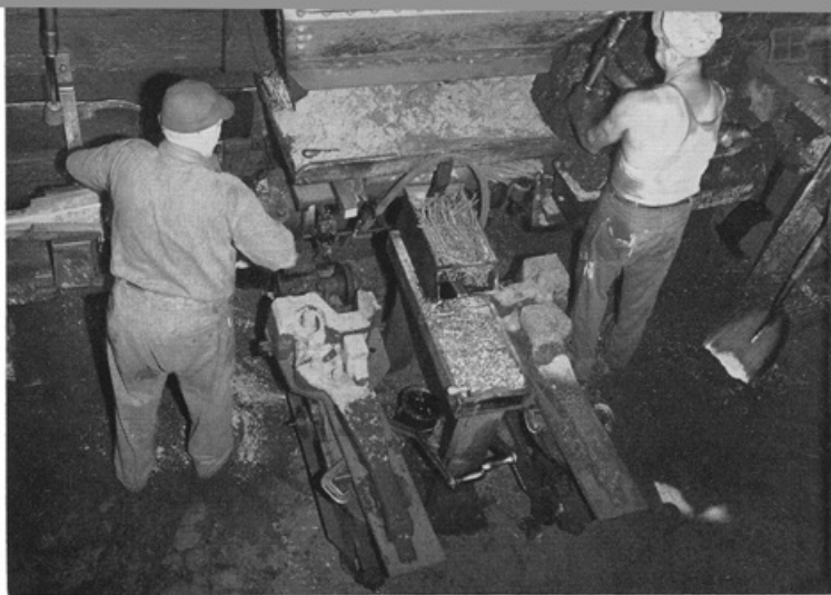
Cores play an essential part in almost all steel castings. Here we see two cores which will be placed back-to-back in a coupler mold. They will form the interior contour of the finished coupler.
