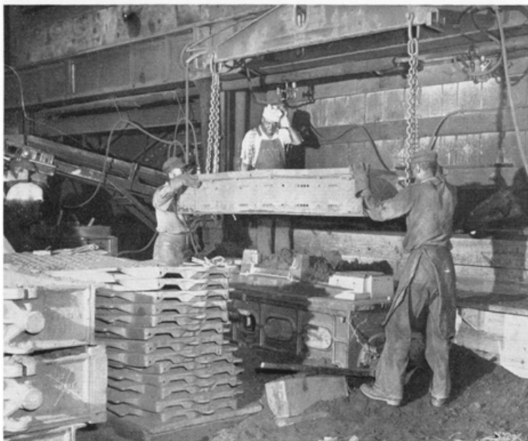
Truck side frame flask being located on pattern preparatory to filling with sand and ramming.
