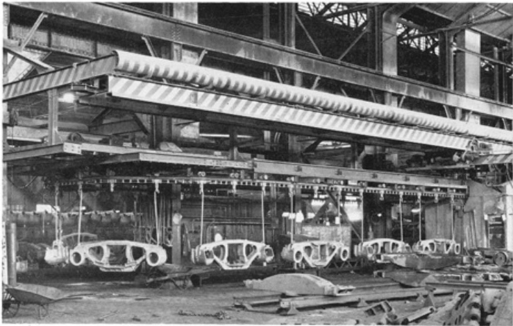
Continuous Shot Blast. Castings are conveyed on an endless chain through an enclosure where high velocity streams of shot remove adhering sand and scale. Compressed air propels the shot through nozzles which are entirely controlled and directed from outside the enclosure.
