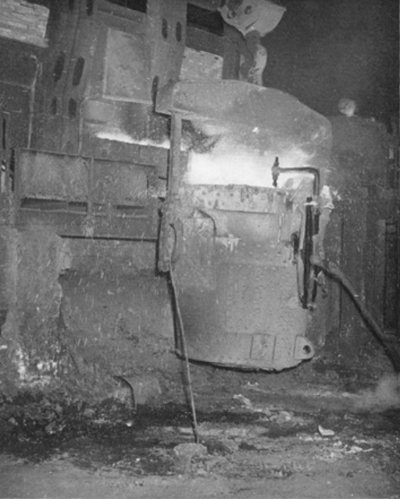
Tapping a heat. This view is on the Foundry side of the furnace and we see 30 tons of molten steel starting to flow from the tap-hole into the ladle. Temperature of the molten steel is close to 3000 degrees.
