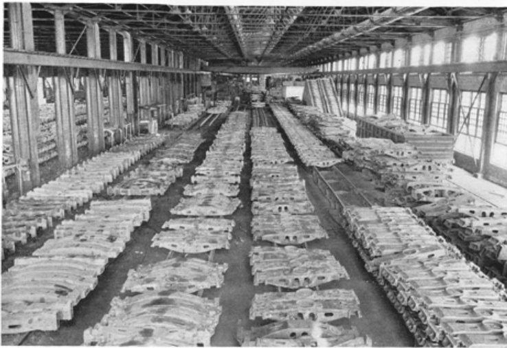
Bolster Finishing Bay. This adjoins the Frame Finishing which may be seen on the left. Heat treating equipment in the Frame and Bolster Finishing Department includes nine car type annealing furnaces and two quench tanks. Either of these tanks could serve as a family size swimming pool — far too deep for wading, however.
