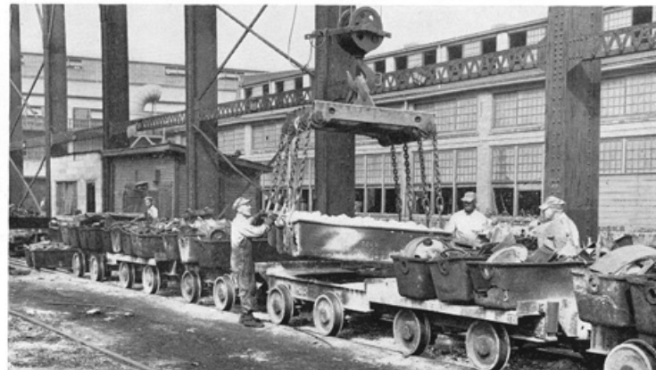
Scrap and pig iron contain impurities which must be removed by a flux or slag. Here a weighed amount of burned lime is included in the furnace charge to form the slag.
