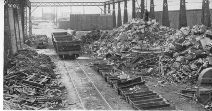
Steel scrap is an essential raw material and comprises three-quarters of the furnace charge, with pig iron as the remaining one-quarter.
