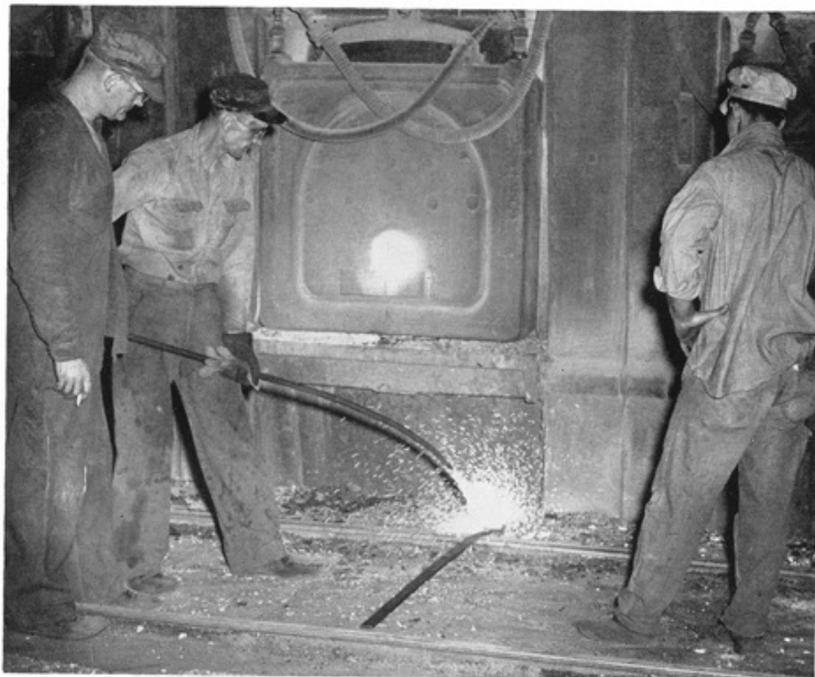
Frequent tests are made during the refining period. One or more will be analyzed in the Laboratory, before final alloy additions are made.
