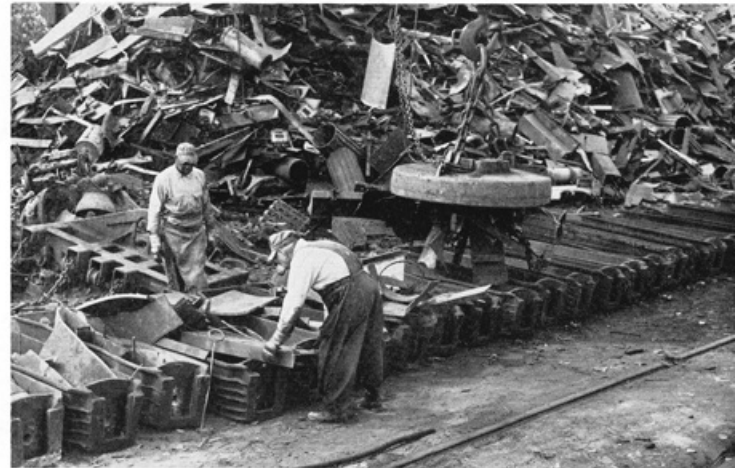
The upper photo shows a part of the scrap storage, while this picture indicates the method of loading charging boxes by magnet.
