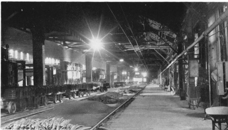
View west along the Open Hearth Platform. Six 30-ton basic furnaces are available to supply molten steel to the Foundry. Producer gas made from coal is used as melting fuel, and each 30-ton heat requires nine tons of coal for this purpose. Waste gases from the furnaces are pulled through boilers and the resulting steam supplies a part of our electric and compressed air power requirements.
