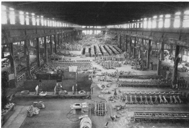
Looking south in Coupler Building. While couplers and draft yokes comprise the largest tonnage finished in this building, many other types of medium and small castings are cleaned and finished here.
